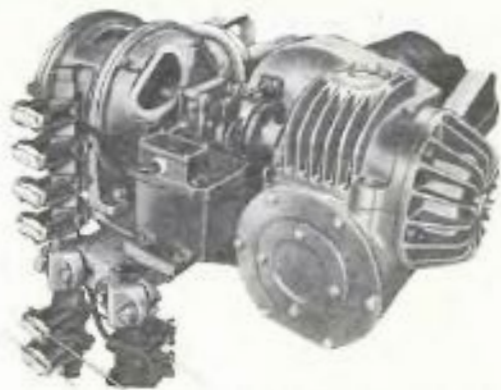
The illustration shows the application of this brake, identified as "Shaw-Box" Type "L," to a worm-driven hoisting unit. Notice the radiating fins on the end of the housing to assist in quickly dissipating the heat.
