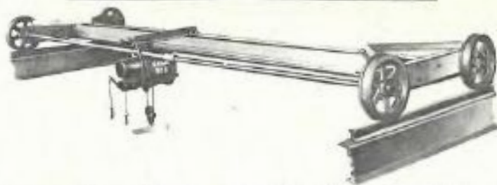
Single point lift push type crane, as used in small ice plants. Bridge and trolley travel is accomplished by pushing on the load. Bridge wheels are of large dimensions to permit fast easy travel. Hoist is heavy duty electric hoist with push type trolley equipped with can dogs instead of the usual hoist hook.
