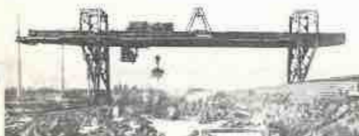
Above illustration is of a magnet handling Gantry Crane with a cantilever at each end, performing a typical rapid handling service. This crane is used to load and unload freight cars in a large scrap yard.
